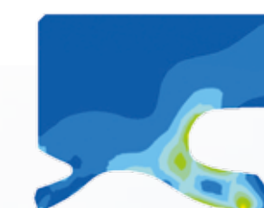
模拟 - 在压力作用下密封件的形变 Simulation - deformation of the seal under pressure
